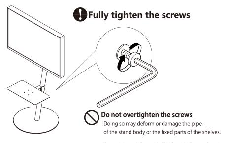
It is not designed to be completely tightened with screws in order to secure it between the pipes.
