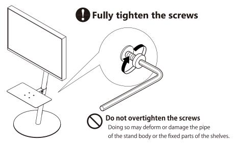
It is not designed to be completely tightened with screws in order to secure it between the pipes.
