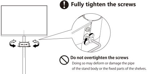
Rotate the mounting part to align it with the front.
