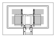
• Depending on the TV specifications (weight / center of gravity) you are using and the mounting position of this product, the overall weight balance may become poor, which may affect the stability of the stand. (When using a small lightweight TV, take measures such as lowering the rack mounting position.)
