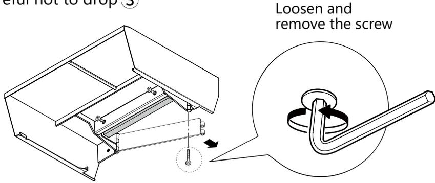
Loosen and remove the screw
