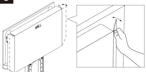
$\triangle$ Forced folding or repeated bending may cause damage.
