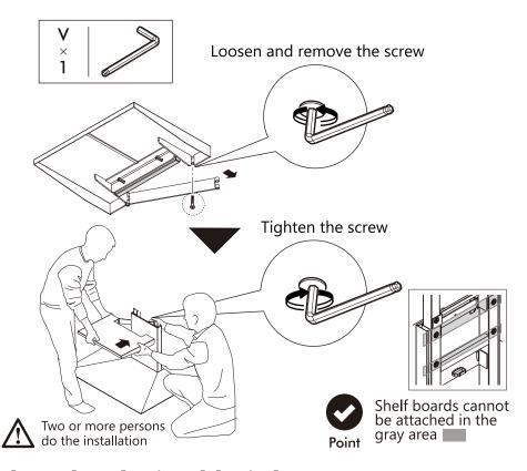
Fix the shelf board at the desired height 3 and fully tighten the screws
