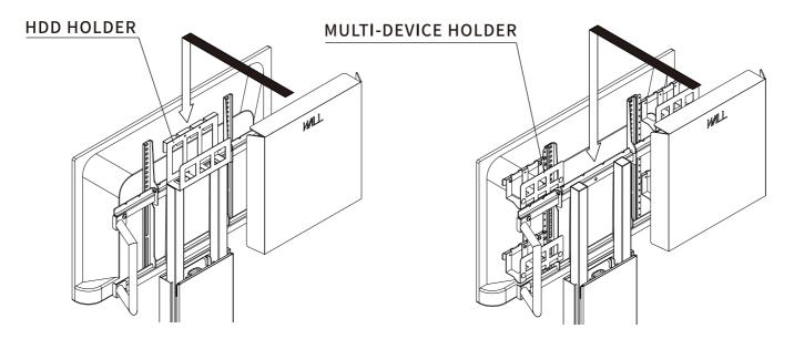
Attach the HDD HOLDER (sold separately) or MULTI-DEVICE HOLDER (sold separately) first, then attach the back cover. If the hooks interfere with HOLDERs, change the direction of the hooks.
