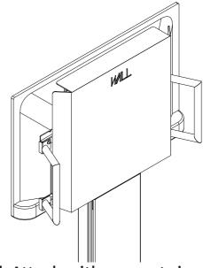
Put the hardware on the top frame of V5
