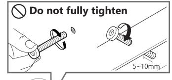
Attach the fixing plate 2 to the shelf plate 1
